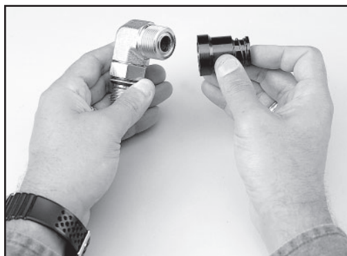
Fig. 21 – O-Ring installation using the CORG assembly tool
